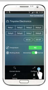
(4) Input your network's settings like SSID, password and IP address in turn, then click "**Start**". The app will send commands to the WiFi module automatically. Click "**Finish**" when the app shows configuration is complete.
