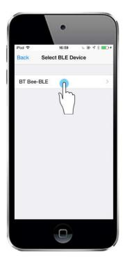
(3) When the app find a device named "BT Bee-BLE", click this device to connect directly
