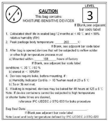
The module Must go through 125°C baking for at least 9 hours before SMT AND IR reflow process!
