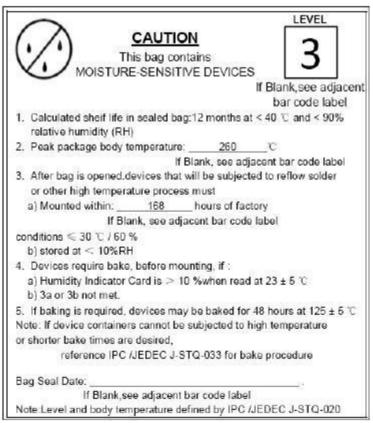
The module Must go through 125°C baking for at least 9 hours before SMT AND IR reflow process!
